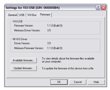
Figure 2-1. VXI-USB Firmware Update Panel
